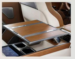
Powered Club Table deploys on a 3D-printed metal support and swivels for either passenger
