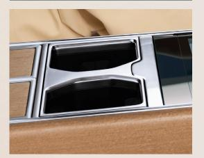
A cam-driven elevator system electrically deploys the flushfitting cup holders
